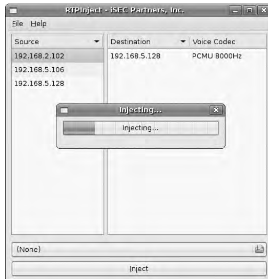
Figure 4-15: RTP injection audio replacement
