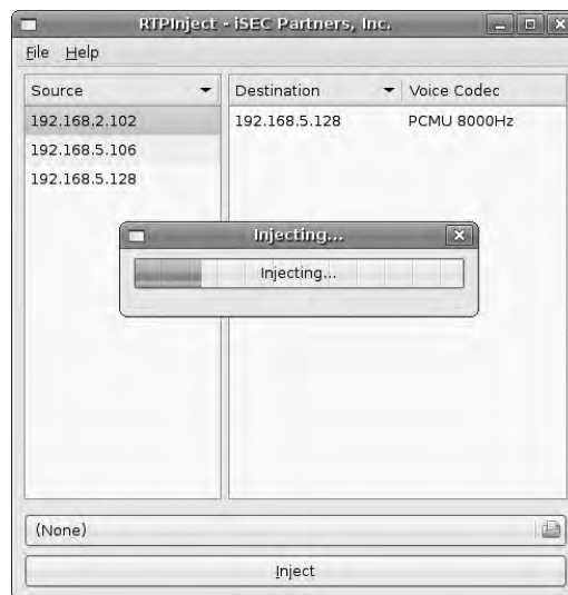
Figure 8-13: Injecting audio with RTPInjct
